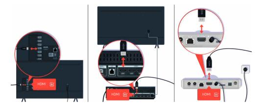
Check the antenna and HDMI cable connections.
