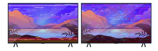
If the issue persists, define exactly what is wrong with the display. For example, mosaics and blocks, multiple lines or white dots or fixed horizontal or vertical lines.
