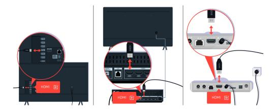
Check the antenna and HDMI cable connections.
