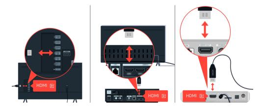
First disconnect and reconnect the power cables and HDMI cables on the back of your TV or the One Connect Box, then unplug the power cable and plug it back into the wall outlet.
