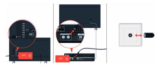
Check the antenna and input cable connections.
