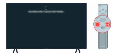
Press the  $\bigcirc$  and  $\bigotimes$  buttons simultaneously to display the pairing animation clip.
