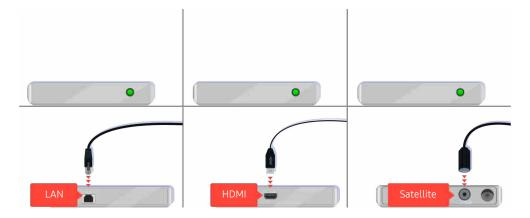
If you are using a set-top box, check the cable connection. The cable you need to check depends on the type of set-top box.
