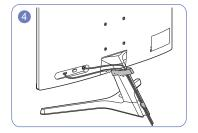
Secure the HOLDER-CABLE to the stand. (HOOK type)
