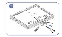
Remove the screws from the bottom of the stand
