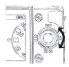
\* For some Sony E cameras, if you set the camera mode dial to A and set the brightness by turning the aperture adjustment ring on the lens, the camera automatically changes the shutter speed. Therefore you don't need to adjust the shutter speed as well, which is required in M mode.
