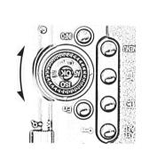
tor the brightness. 2) Adjust the shutter speed by turning the dial to achieve the appropriate exposure
