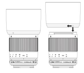
Align the attachment reference point on the hood with the reference point on the lens. Push the hood onto the lens and turn the hood to the right until it makes a clicking sound.
