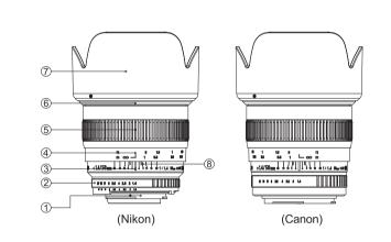
1 Mount (camera locking area) 4 Focus scaling ring 7 Hood
