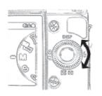
\*\* For some Sony E cameras, if you set the camera mode dial to A and set the brightness by turning the aperture ring on the lens, the camera automatically changes the shutter speed. Therefore you don't need to adjust the shutter speed as well, which is required in M mode.
