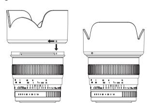
Align the attachment reference point on the hood with the reference point for a hood on the lens, push the hood onto the lens and turn the hood to the right until it makes a clicking sound.
