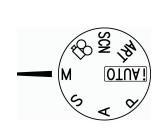
2) Adjust the shutter speed by turning the dial to achieve the appropriate exposure for the brightness.
