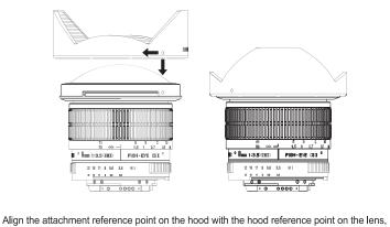
push the hood onto the lens and turn the hood clockwise until it makes a clicking sound.
