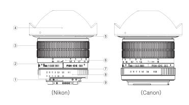
① Mount (camera locking area) ② Distance scale point ⑤ Hood locking tube Point ring ® Aperture adjustment ring ® CPU (electronic contact)
