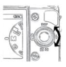
\*\* For some Sony E cameras, if you set the camera mode dial to A and set the brightness by turning the aperture adjustment ring on the lens, the camera automatically changes the shutter speed. Therefore you don't need to adjust the shutter speed as well, which is required in M mode.
