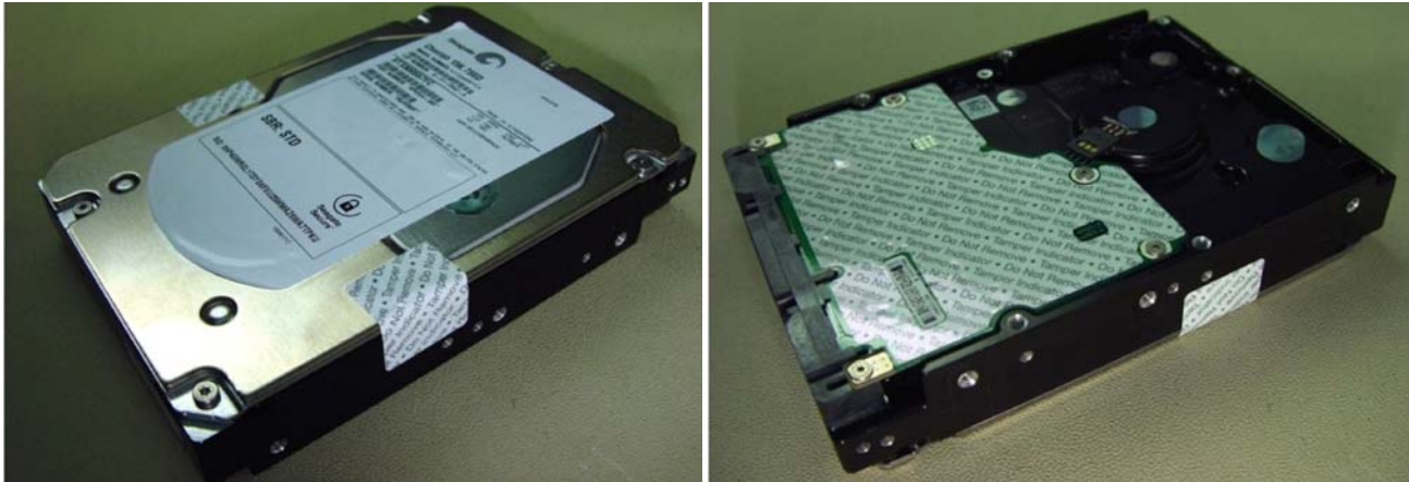
Figure 7. Example of FIPS tamper evidence labels.
