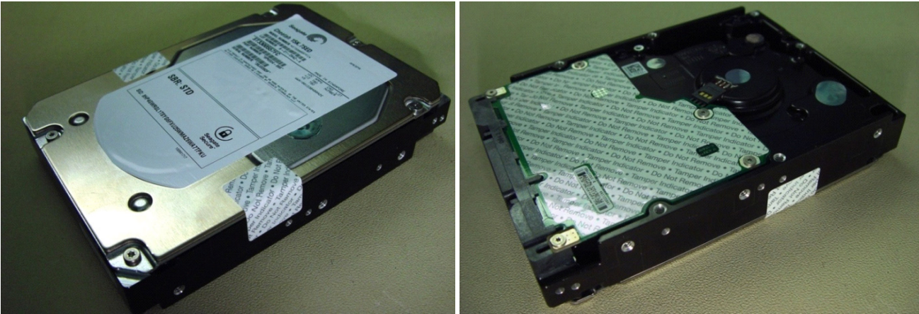
Figure 7. Example of FIPS tamper evidence labels.
