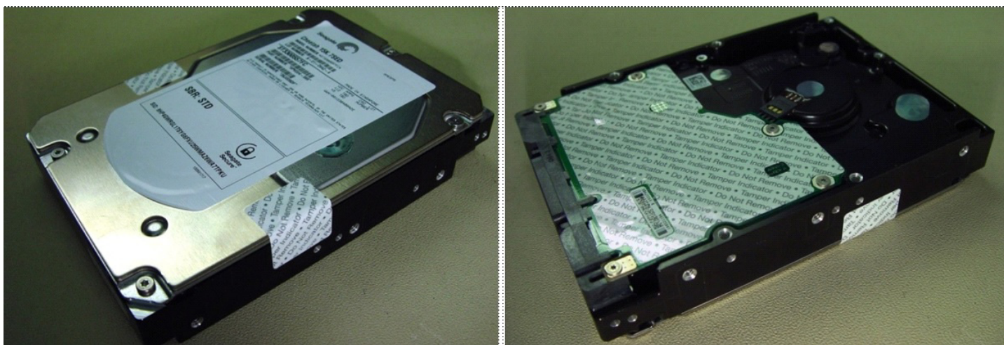
Figure 4. Example of FIPS tamper evidence labels.
