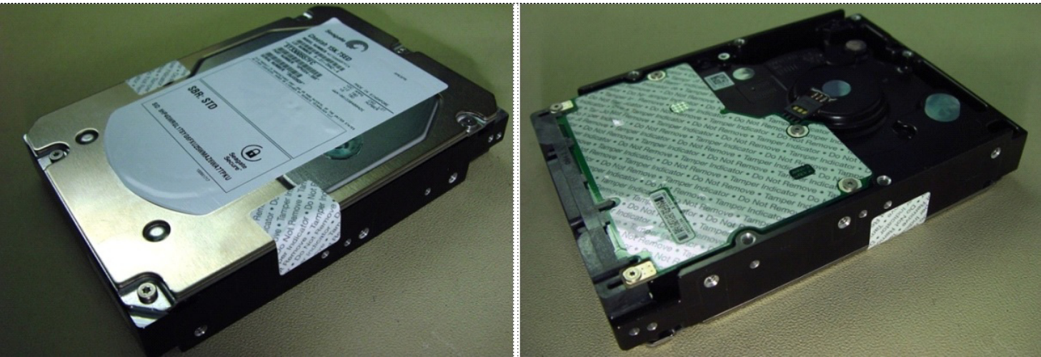
Figure 8. Example of FIPS tamper evidence labels.
