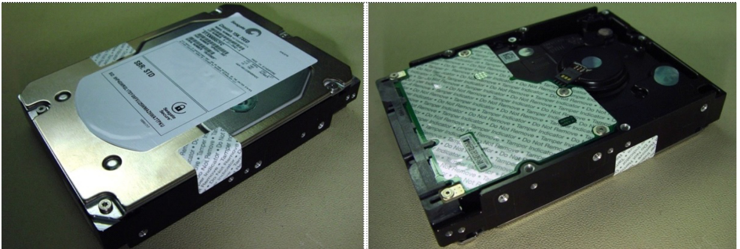
Figure 10. Example of FIPS tamper evidence labels.
