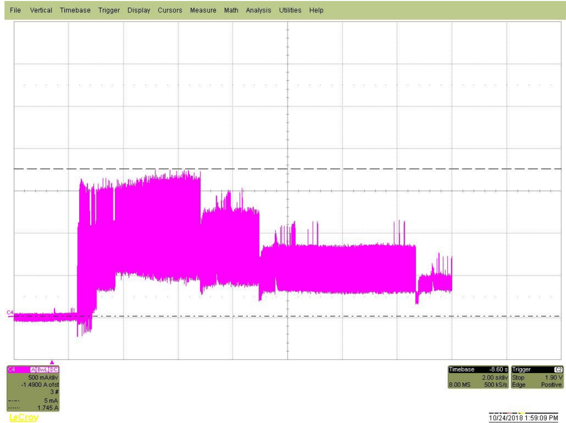
Figure 1. Typical 12V startup and operation current profile
