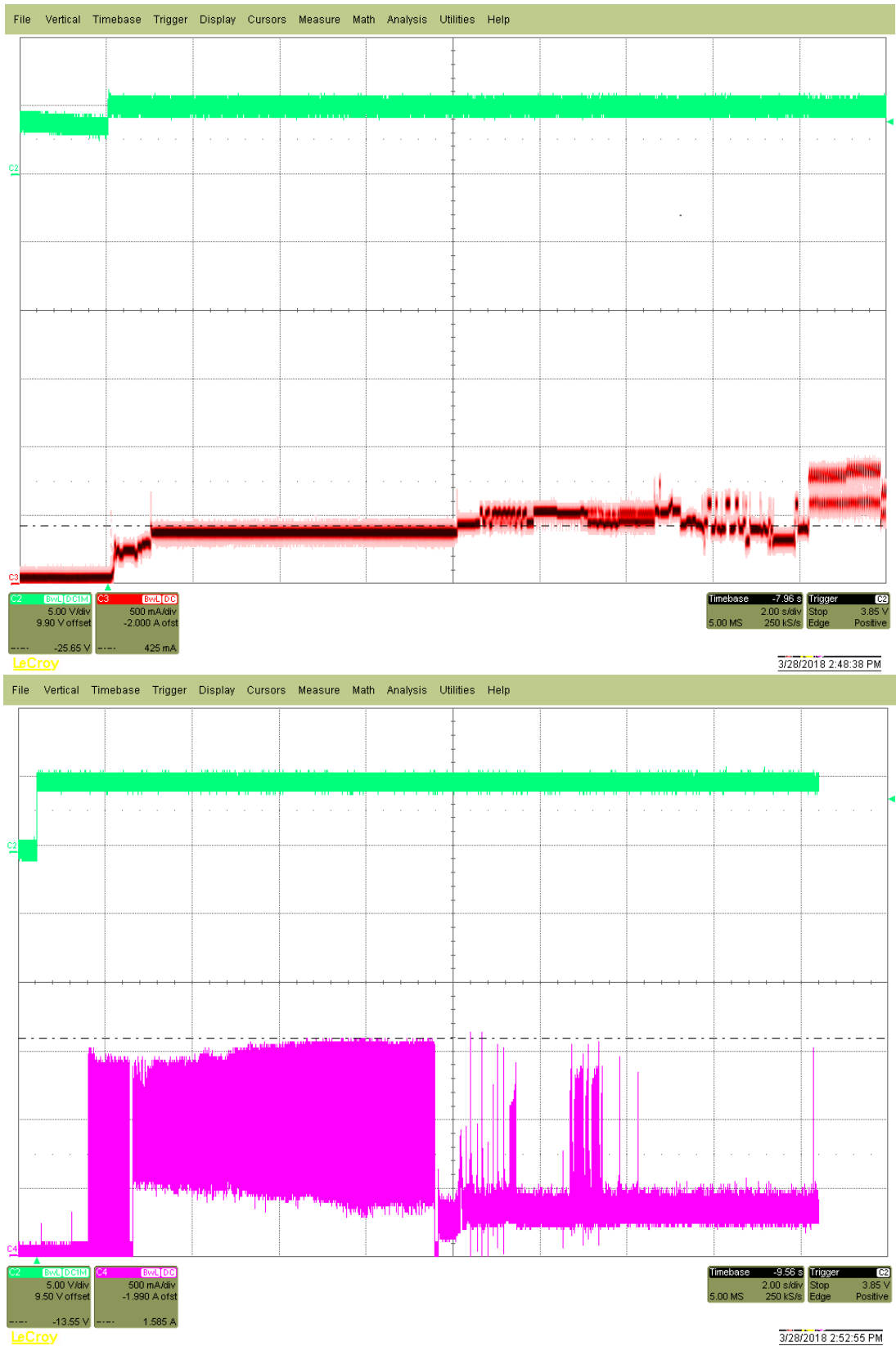
Figure 2. Typical 5V and 12V startup and operation current profiles (14TB, 12TB and 10TB)
