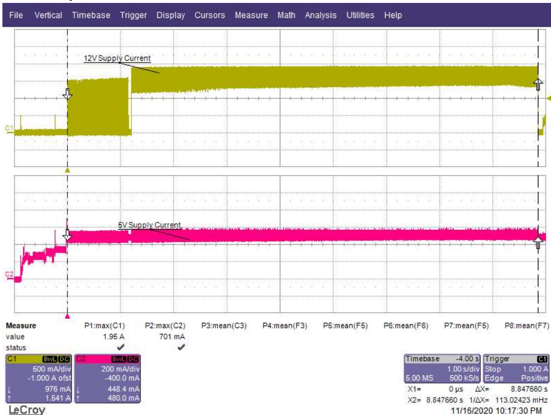
Figure 1. Typical 12V startup and operation current profile
