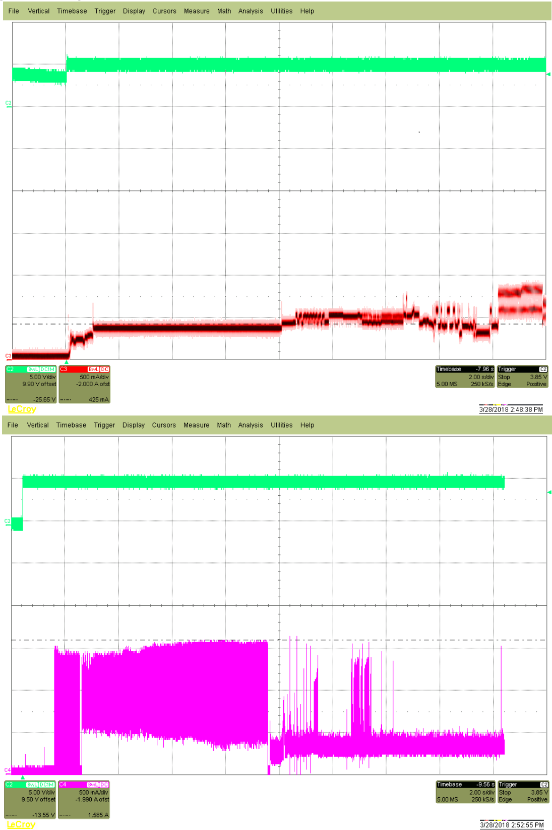
Figure 1. Typical 5V and 12V startup and operation current profiles
