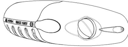
Place it in a central position to set an optimal temperature for normal use. The more you turn the knob clockwise, the lower the temperature in the refrigerator will be. The more you turn the knob counterclockwise, the higher the temperature in the refrigerator will be.
