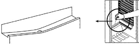
Make sure that the drain gully and the drain opening are not blocked so that the water produced in the refrigerator can always flow off unobstructed.
