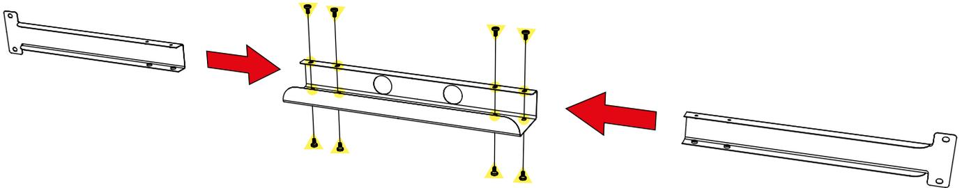
**EN** Screw together the three parts of the cable management system with eight M6 screws (B) using the hex key (D).
