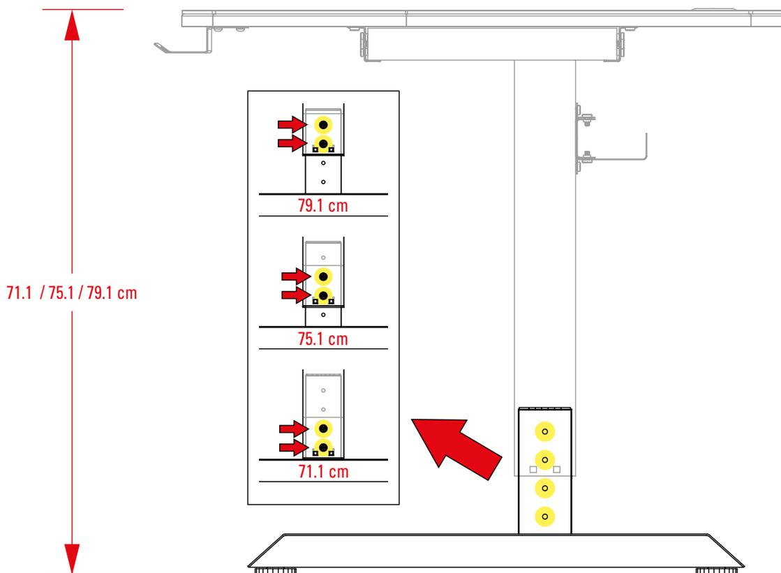
**EN** The desk can be adjusted to three heights during assembly: 71.1 cm, 75.1 cm and 79.1 cm. Place the screws one hole higher to position the tabletop higher up and one hole lower to position the tabletop lower down.
