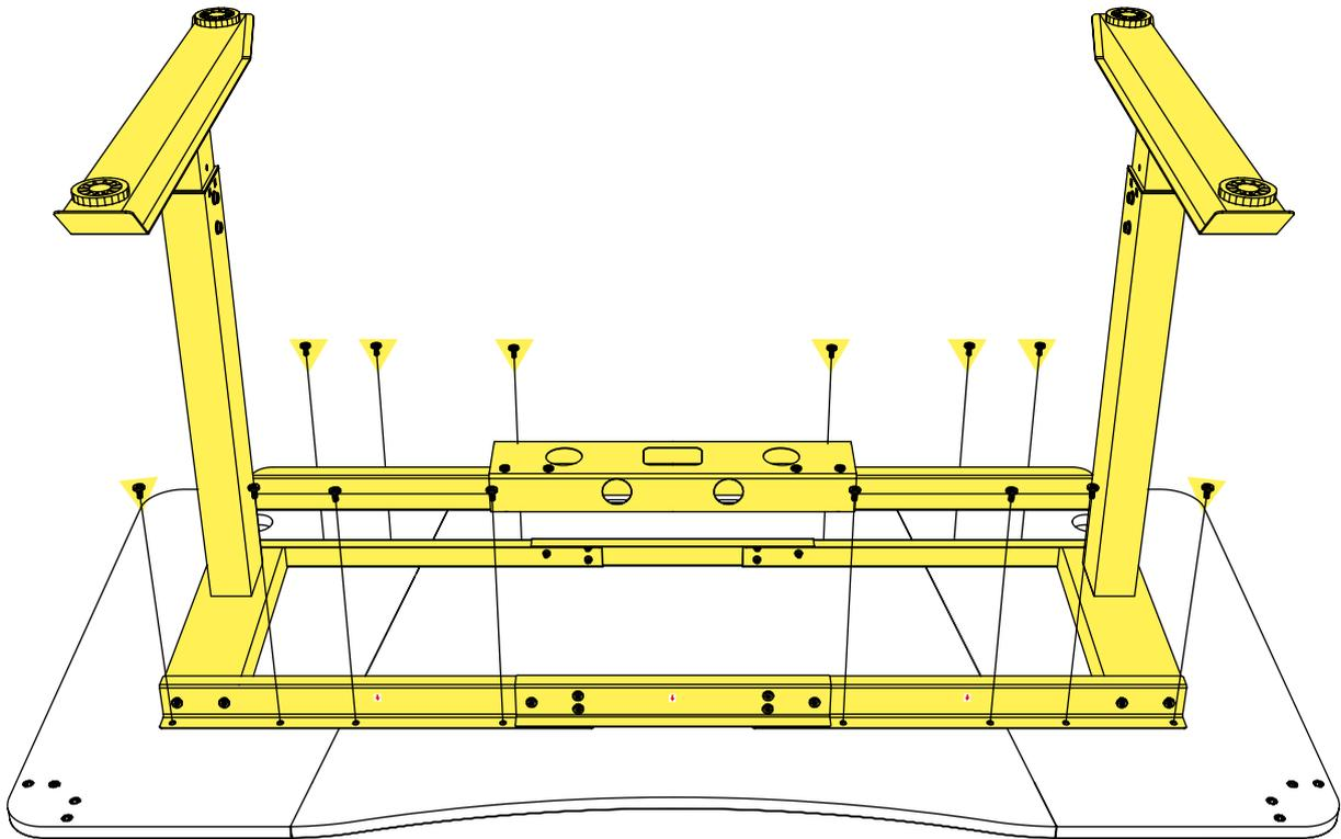
**EN** Attach the desk frame to the tabletop with 16 M6 screws (B) using the hex key (D).
