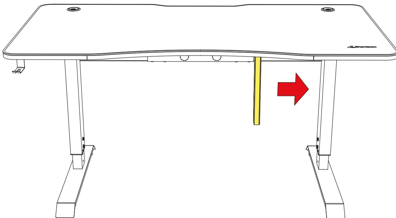
**EN** Attach the magnetic cable channel (I) to the left or right desk leg.
