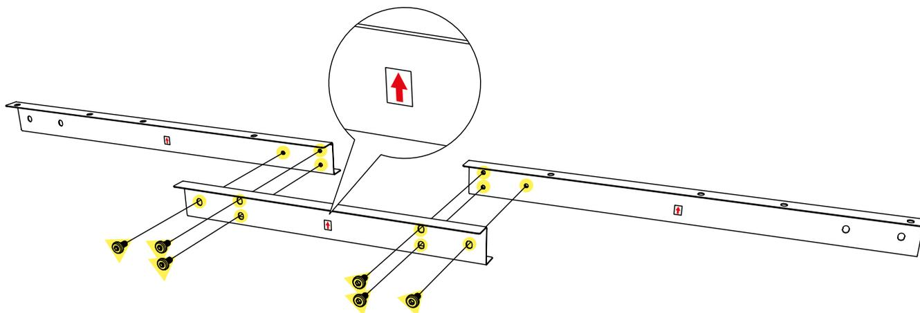
**EN** Use the hex key (D) and six M6 screws (B) to screw the beams together. **Attention: Make sure that the beam parts are assembled correctly and with the red arrows pointing upwards! Only tighten the screws completely after the desk frame has been correctly positioned on the tabletop.**
