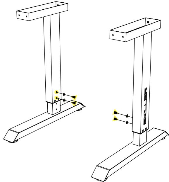
**EN** Place a washer (C) on each of the four M8 screws (A). Then screw the two legs onto the desk feet, each with two screws (A) using the hex key (D).
