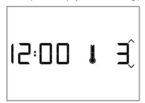
After starting operation, the thermometer on the right next to the time display shows the heating up progress of the interior temperature. The thermometer gradually lights up as the appliance heats up. When the thermometer is fully lit, the appliance has reached the set temperature. When using the grill, the thermometer is fully lit immediately.
