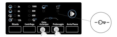
If pressed any button while child lock is active, the Additional Function Leds will blink on the display.
