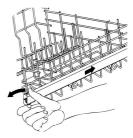
Version B: with adjustment in three positions on both sides.
