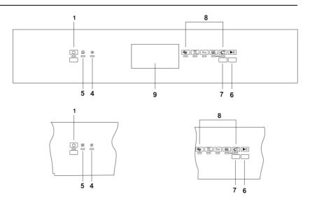
**ON/OFF** BUTTON AND WARNING LIGHT 2 Not present 3 Not present **SALT WARNIN LIGHT** 4 **NO RINSE AID LIGHT** 6 **PROGRAM SELECTION BUTTONS** START/PAUSE BUTTON 7 8 **PROGRAM INDICATOR LIGHTS** HANDLE TO OPEN THE DOOR 9
