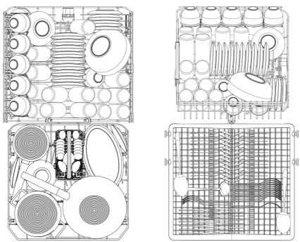
If the bottom basket inserts are of the fold-down type, they should be laid flat for easier loading.
