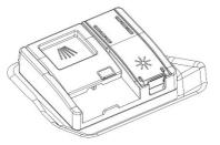
The rinse aid helps the dishes dry faster and prevents the formation of scale deposits and staining; it is automatically added to the water during the final rinse cycle, from the container situated on the inner side of the door.
