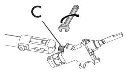
2. Use a spanner to remove the nozzles "C" and install the new ones for the required gas supply, following the indications given in the relevant table (see "Gas types and Countries").
