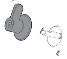
3. Remove the flame-spreader crowns and relative burner caps.
