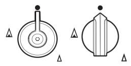
Used for lighting and adjusting the hob burners. Press and turn anti-clockwise to  $\Lambda$ in order to light the relative burners. Turn the knobs to the zone between the maximum  $\Delta$  and minimum  $\Delta$  setting to adjust the flame. Return the knobs to the position to turn off the burners.
