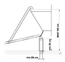
It is important to prevent the hose from coming loose and falling. For this purpose, the plastic support is equipped with a hole for tying it to the wall or water tap. The free end should be positioned at a height of between **30 and 100 cm**, and should never be submerged in water. If a horizontal drain extension hose is used (for a maximum 3 m), the drain hose can be placed at a maximum height of **.85 cm** from the ground.
