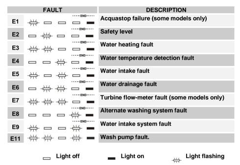
If an alarm occurs, the machine stops the current program and indicates the fault.
