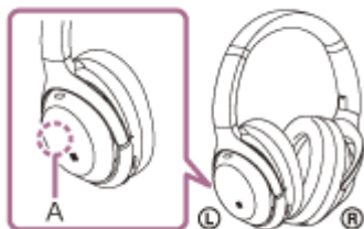
A: Location of the built-in antenna
