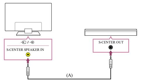
(A) TV centre speaker mode cable (supplied with devices such as sound bars that have S-CENTER OUT terminals)
