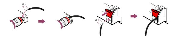
\*Strip about 10 mm (13/32 inches) of insulation from the speaker cable at each end.
