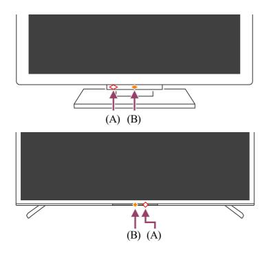
(A) Voice function LED (On the left side or centre right at the bottom of the TV. Only TVs with a built-in MIC.\*)
