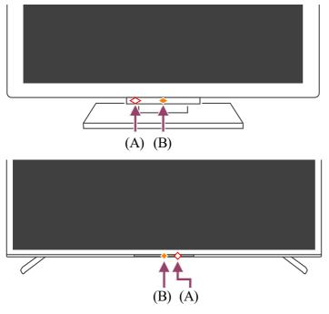
(A) The voice function LED is located at the bottom just left of centre or centre right of the TV.(B) The LED located at the bottom centre of the TV lights up amber when the TV is set to detect "Ok Google".
