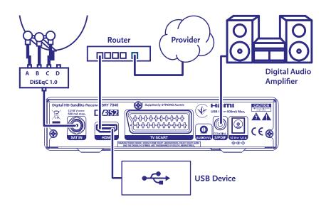
This port can be used for USB storage devices such as USB pen drives or HDD with a maximum peak current of 500 mA. It is recommended to use USB 2.0 storage devices for playback of video files or HD movies.
