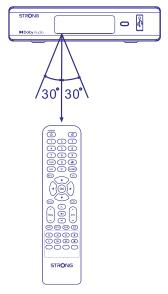
To use the remote control, point it towards the front of the digital receiver. The remote control has a range of up to 7 metres from the receiver, if properly aligned towards the IR eye on the front panel. The remote control will not operate if its path is blocked.
