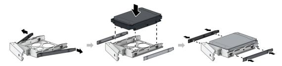
• For 2.5" drives: Remove the fastening panels from the sides of the drive tray and store them in a safe place. Place the drive in the area of the drive tray indicated below. Turn the tray upside down and tighten the screws to secure the drive in place.
