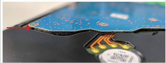
Missing insulator (insulation sheet)
