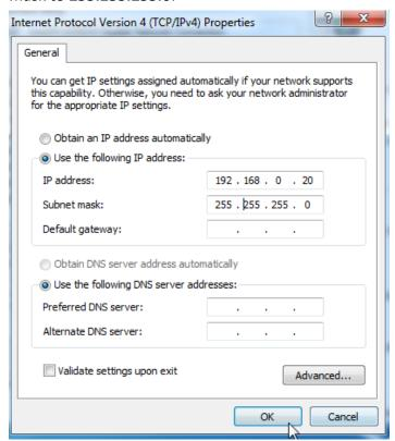
Step 3 Start a browser (such as Chrome) and enter the IP address of the switch (default: **192.168.0.1**) in the address bar to access the login page.
