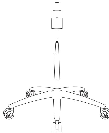
3. Place the chair face down and insert the star base into the butterfly mechanism.
