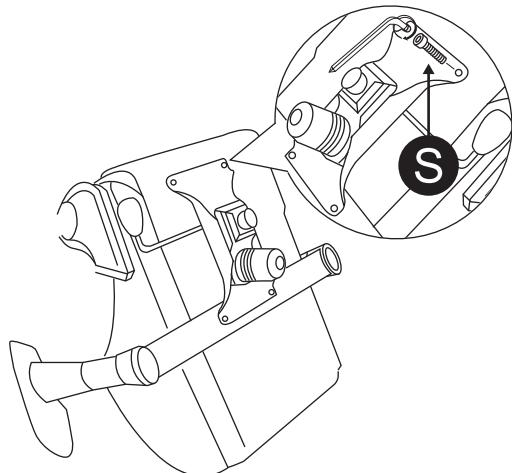
NOTE : Place the screws by hand before tightening them in an X-Pattern with the allen key.
