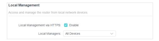
• Allow all LAN connected devices to manage the router:
