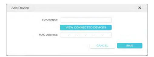
3. Click VIEW CONNECTED DEVICES and select the device to manage the router from the Connected Devices list, or enter the MAC address of the device manually.
