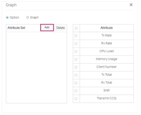
3. In the pop-up window, specify a name for the template and select the information options which will be displayed in the graph. For example, we specify the template name as Graph-1, and select CPU Load, Client Number and SNR to be displayed. Click **OK**.
