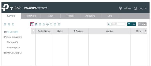
2. In the pop-up window, select your desired scanning method, and click **OK**. There are two methods provided: **Auto** and **Custom IP-Range Scan**. With **Auto** selected, Pharos Control will scan the devices in the same subnet. With **Custom IP-Range Scan** selected, you can specify the IP range of the devices, and Pharos Control will scan the devices in the IP range. **Custom IP-Range Scan** should be selected if you want to scan the devices in a different subnet.
