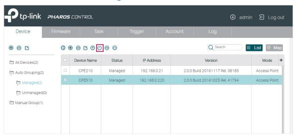
2. In the pop-up window, verify the device to be rebooted and click **OK**. Wait for a moment and the device will reboot automatically.
