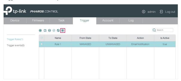
5. After all the configurations above are completed, you can use this feature without any other operations. If needed, you can also manage the trigger rules and view the trigger events on the this page.
