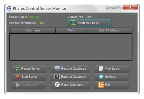
The upper half of the window displays the running status of Pharos Control. The lower half contains corresponding operation buttons. For details, refer to the following table:
