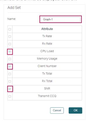
4. The template is created. You can add more templates or delete the unused templates on this page. Also, you can edit the displayed information options in the right-hand column by checking or unchecking the boxes.
