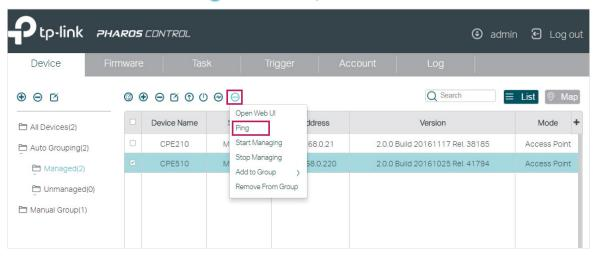
2. In the pop-up window, set the number of ping packets to be sent and the timeout value. Timeout value determines how long Pharos Control will wait for the response from the device before the ping is regarded as failed. Click **Start to Ping**.
