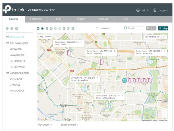
All devices are on the map. You can drag these devices to the appropriate locations according to their actual locations. Also, you can select one or more devices on the map, and do the operations introduced in the above sections, such as group the devices, view the graphic data information of the devices, and upgrade, ping, and reboot the devices.
