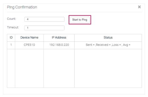
3. View the ping result in the Status column. As the following figure shows, Pharos Control sent 4 ping packets to the device and a response was received from the device every time, which indicates that the connection between Pharos Control and the device is normal.
