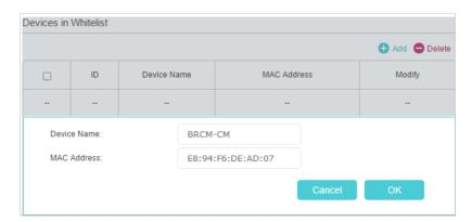
Enter the Device Name and MAC Address. (You can copy and paste the information from Online Devices table if the device is connected to your network.)
