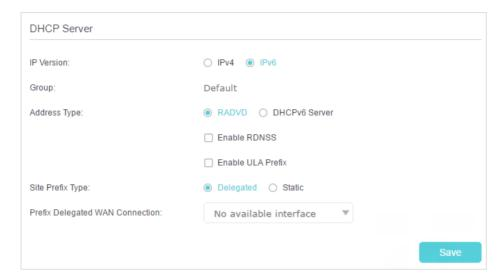
13) Select the RADVD address type to make the modem router assign IPv6 address prefixes to hosts.
