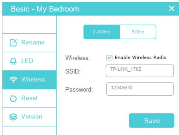
3. Keep the [Enable Wireless Radio](#) checkbox selected, enter a new SSID and password, and click [Save](#).
