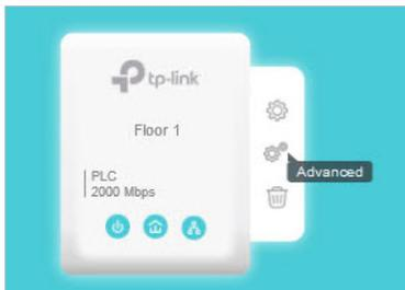
2. Go to the **Mode** page and enable **Lower PLC-to-VDSL Interference Mode**.
