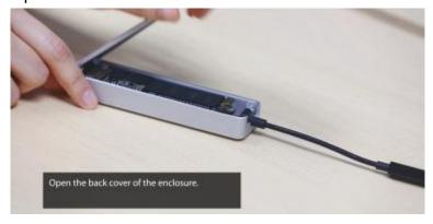
**Step 4**Use the T5 screwdriver to remove the screw holding the JetDrive SSD.
