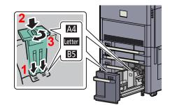
Make sure that the top of the paper size guide (A) matches the paper size to be used, attach the clamp, and rotate the clamp to lock it.
