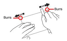
Before loading Hagaki into the multi purpose tray, fan them and align the edges. If the Hagaki paper is curled, straighten it before loading. Printing onto curled Hagaki may cause jams.
