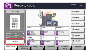
The machine starts scanning the original. When scanning is completed, the preview image appears on the panel.
