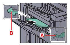
two points, place the paper with the center aligned to the center point between the two side guides (A and B).
