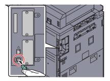
**3** Insert the cord into the groove.
