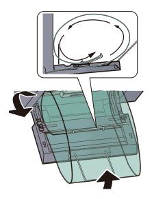
4 Adjust the paper width guides to the width of the paper.
