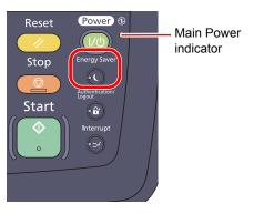
If print data is received during Low Power Mode, the machine automatically wakes up and starts printing. Also when fax data arrives while the machine is in Low Power Mode when using the optional fax, the machine automatically wakes up and starts printing.
