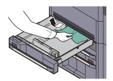
To remove paper which is difficult to get access to, the inner part of the cassette can be removed.
