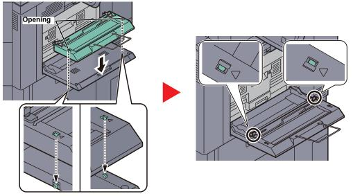
Fit the openings on the sides of the banner tray onto the tabs on the sides of the multi purpose tray, and press into place.
