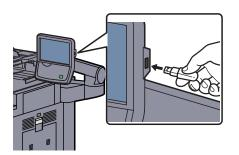
When the machine reads the USB memory, "Removable Memory is recognized. Displaying files. Are you sure?" may appear. Press [Yes] to display the removable memory screen.
