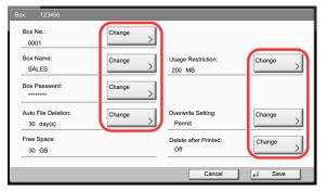
To edit details, press [Change] of the detail you wish to edit. Edit the detail as desired and press [OK].
