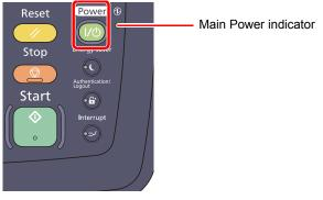
Press the [Power] key. The [Power] key light will go out, and the Main Power indicator will light up.
