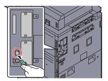
**3** Insert the cord into the groove.
