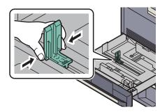
2 Press the (Paper Width Guide) Lock to release the lock. Grasp the paper width adjusting tab and move the paper width guides to fit the paper.
