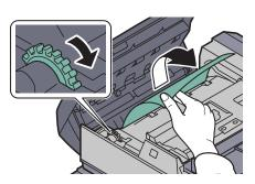
If the original is difficult to remove, turn the dial. The original will scroll out to a position where it can be removed easily.
