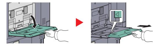
When loading paper sizes 12 x 18" and from A3 to B4 and Ledger to Legal, extend the support tray section of the multi purpose tray until the " $\Delta$ " mark is fully appeared.
