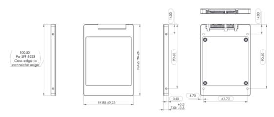
The figure below is enlarged to show detail, but is not the actual size of the form factor. This figure shows 2.5"/7mm cased one-half form factor (for 250GB and 512GB capacities only).
