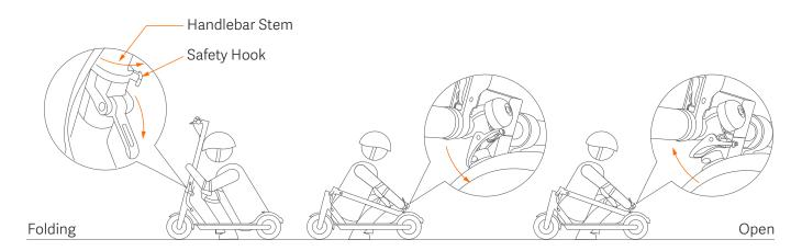
The scooter needs to be turned off before folding. Hold the handlebar stem, turn it counterclockwise to open the safety hook and open the quick release lever. Align the bell and the buckle and hook them. When opening, disengage the bell lever from the buckle on the mudguard. Fold the handlebar stem up, close the quick release lever and turn the handlebar stem clockwise to close the safety hook.
