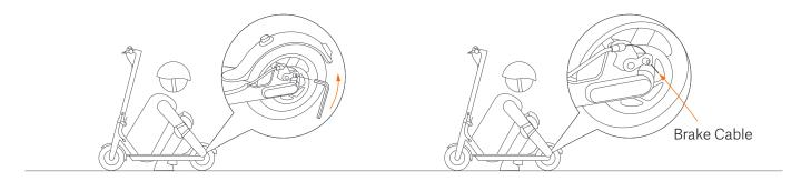
If the brake is too tight, use the 4 mm Allen key to loosen the screw on the caliper. Then slightly adjust the brake line (decrease the exposed length), and tighten the screw again.
