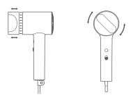
WARNING: Please install the air nozzle while the hair dryer is turned off. Do not adjust or remove the air nozzle during use to avoid getting scalded.
