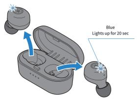
If the earphones do not automatically connect to a Bluetooth device, they are waiting for a connection or are in pairing standby mode. Make the connection to the earphones from your Bluetooth device.
