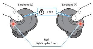
• When the remaining battery power of the charging case is depleted, the earphones will not turn off even when they are placed in the charging case. If this happens, use the function keys on each earphone to turn them off.
