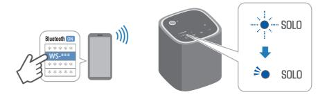
When the connection is established, the SOLO lamp glows blue.
