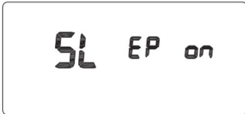
SE oF 3 30/15 60/30 120: Keeping idle for 3/15/30 minutes will enter the dormancy state and 30/60/120 minutes will shut down the speedlite.
