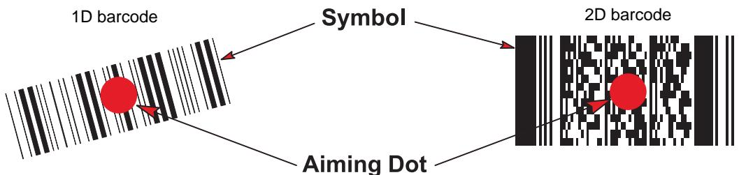
The digital scanner can also read a barcode presented within the aiming dot not centered. The top examples in [Figure](#) show acceptable aiming options, while the bottom examples can not be decoded.
