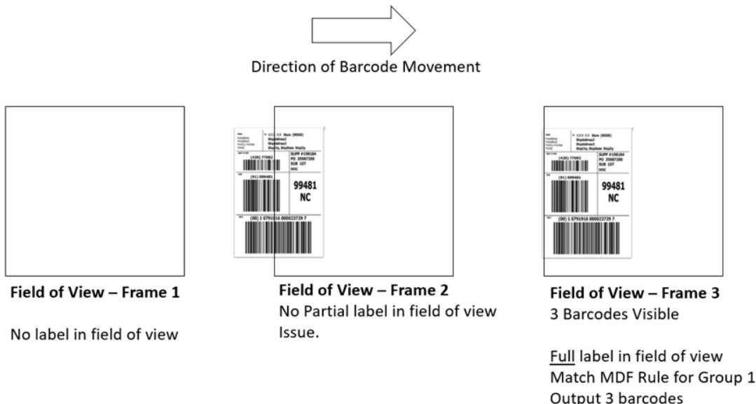
**Figure 20** Scanning Label in a Vertical Orientation
