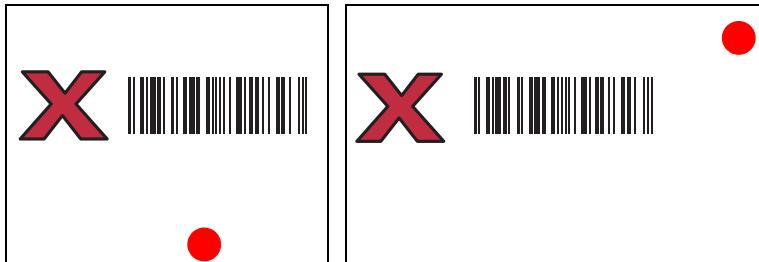
The aiming dot is smaller when the digital scanner is closer to the symbol and larger when it is farther from the symbol. Scan symbols with smaller bars or elements (mil size) closer to the digital scanner, and those with larger bars or elements (mil size) farther from the digital scanner.
