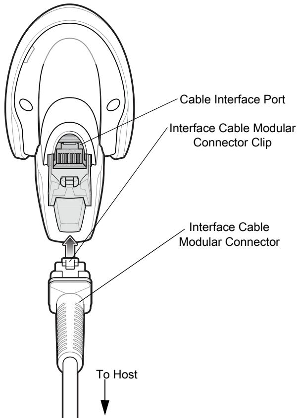
2. Gently tug the cable to ensure the connector is secure.
