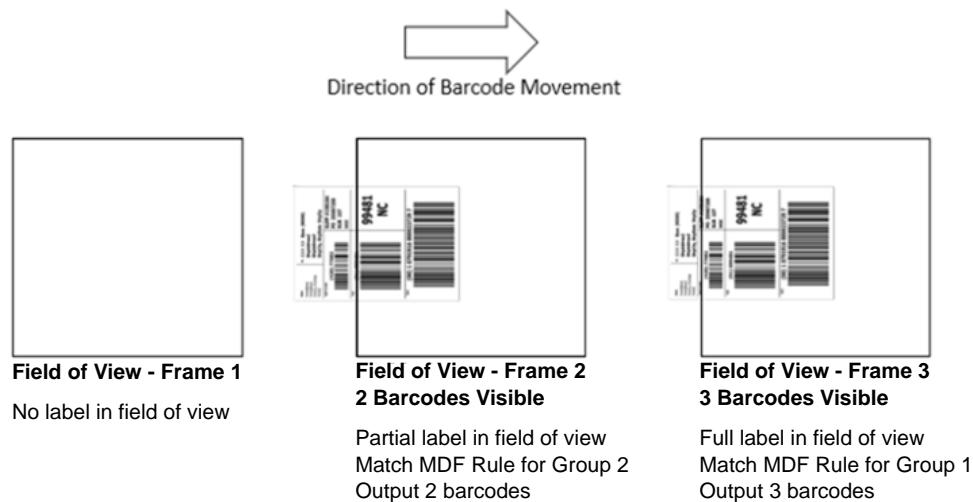
**Figure 19** Scanning Label in a Horizontal Orientation
