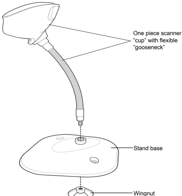
2. Fit the bottom of the gooseneck piece into the opening on the top of the stand base.
