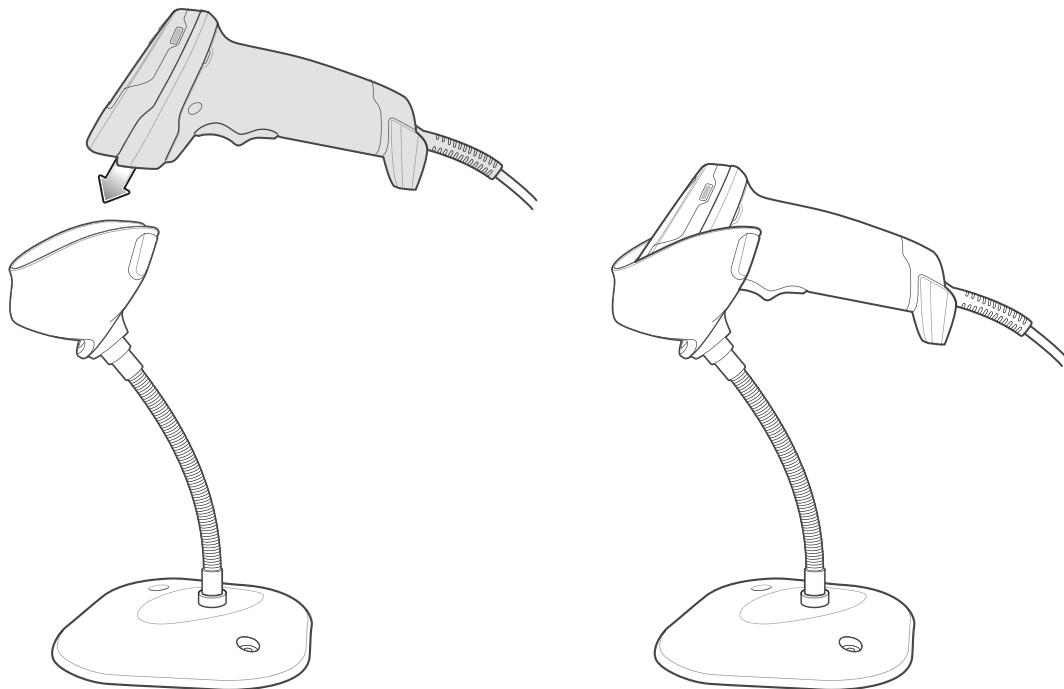
3. Adjust the scan angle by bending the stand's flexible "gooseneck" body.
