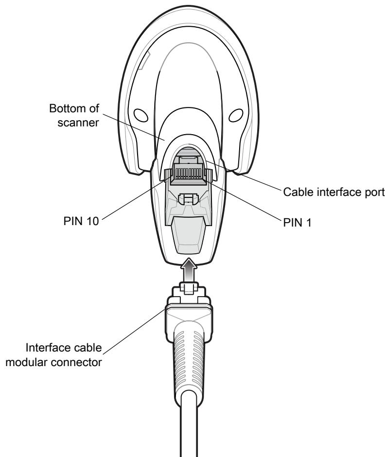
The signal descriptions in [Table 11](#) apply to the connectors on the DS4608 imaging scanner and are for reference only.
