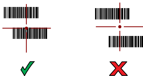
Figure 24 RS6000 Pick List Mode with Multiple Barcodes in Aiming Pattern
