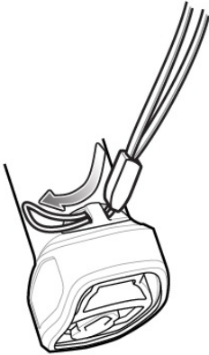
Figure 1-20 Insert Lanyard Loop
