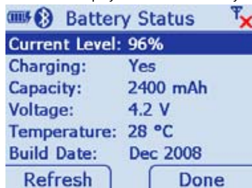
Figure 2-9 Battery Status Screen
